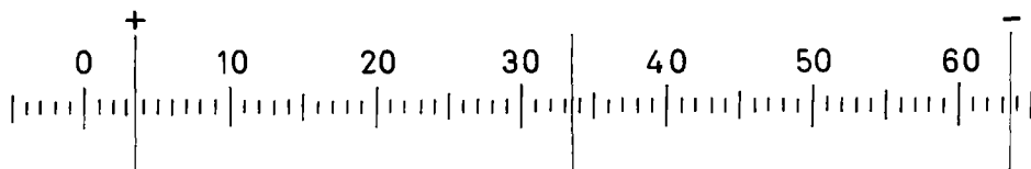
FIG. 17. Eyepiece scale of field balance.
