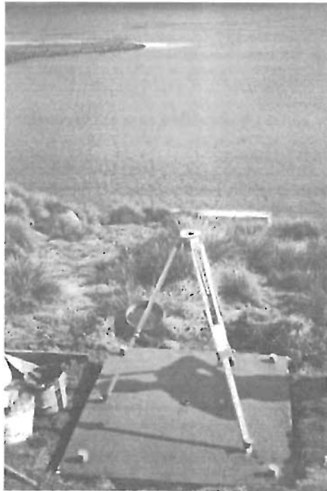
Figure 4.4 French repeat station at Ile Saint Paul, at which a slab has been constructed to support the tripod.
